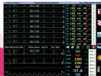
The *Omniview*® gives a real time display of all patient vital signs: *Heart rate, Last BP reading, SpO<sub>2</sub>, Temp, EtCO<sub>2</sub> and Respiration rate.*
