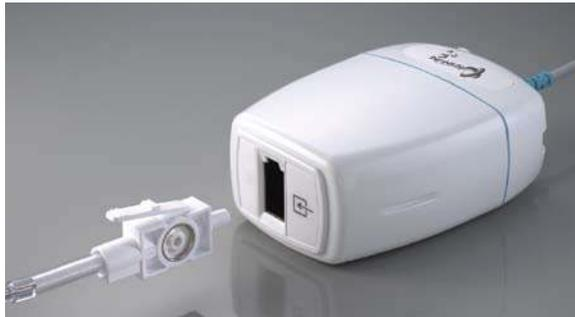
The Infinium *Capnotrac*<sup>®</sup> module is a field upgradable plug in module that can measure End-tidal CO<sub>2</sub> alone or End-tidal CO<sub>2</sub> with, O<sub>2</sub>, N<sub>2</sub>O, Halothane, Sevoflurane, Desflurane, Enflurane and Isoflurane gasses.
